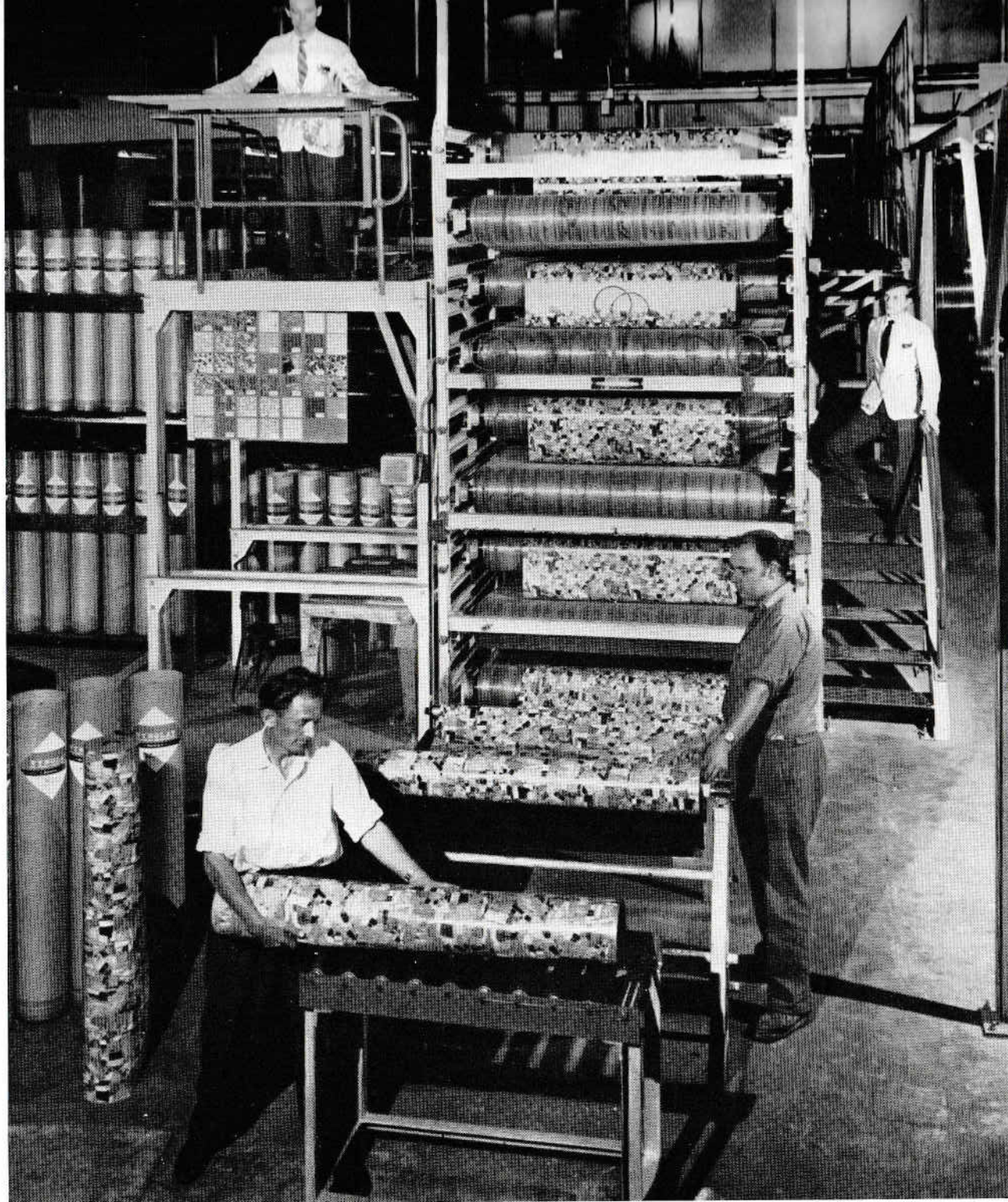
The last stage of Dunlop Vynolay manufacture during which the material is annealed
